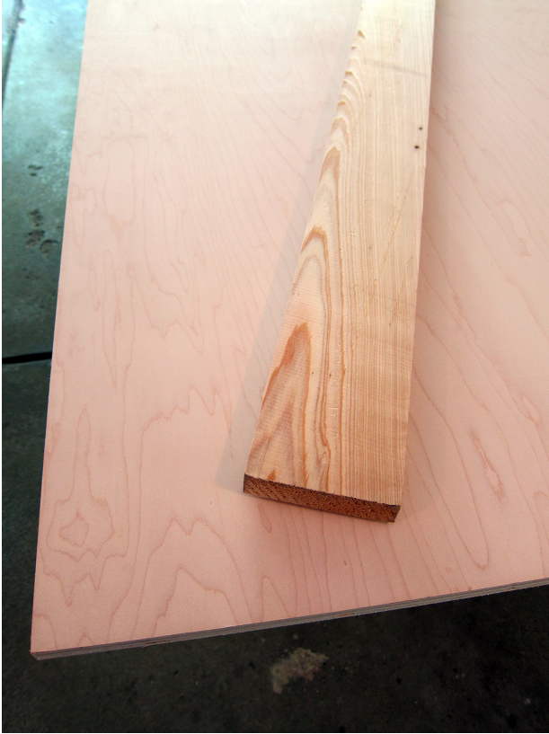
▲ Material List: \frac{3}{4} " thick maple veneer plywood with solid cypress edge-banding. Cut plywood into 4 pieces: top, shelf, and 2-piece "strut" to support the table.
