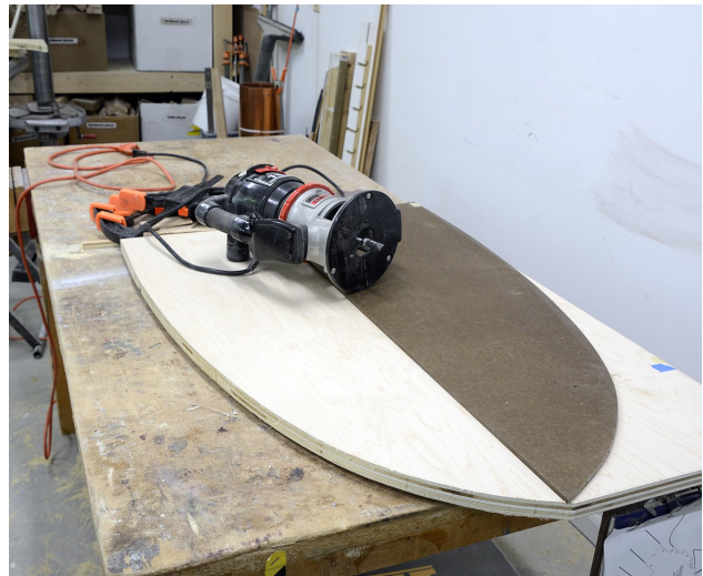
▲ The rough-cut curved Pod top & shelf were made using a band-saw; and then fine-tuned FLW's distinctive curved shape using router with straight flush trim bit. The trimmed top became the "template" to cut Wright's "facia" support shown on pg.3 ...
